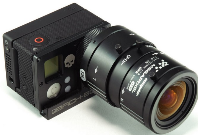
Figure 3. Modified GoPro Camera with Attached Zoom Lens
