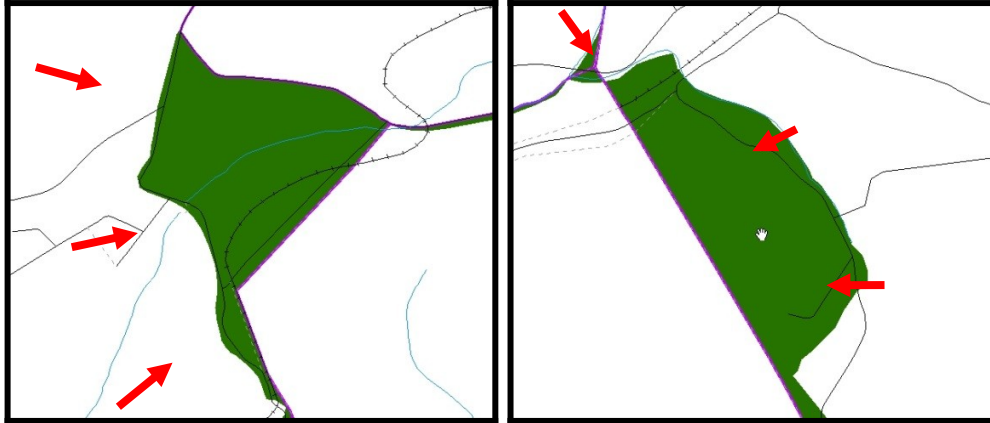
Figure 39. Polygons That Should Be Snapped to Roads or Rivers
