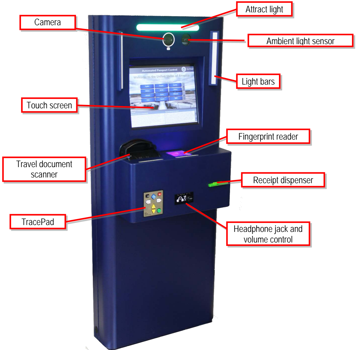
Figure 1: Standard Kiosk Components
