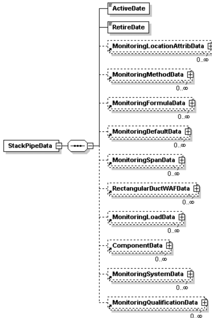
Figure 6 STACK PIPE DATA Elements
