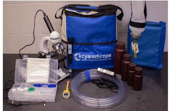
Figure 8: Cyanobacteria monitoring kit & components
