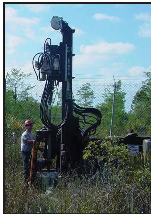
In other areas such as Big Cypress National Preserve, operators have used sonic drilling technologies to drill shotholes which eliminated drill cuttings on the surface that must later be cleaned up.
