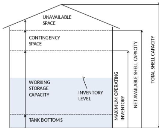
**Figure 2. Schematic of Cavern Storage Capacity and Stocks**
