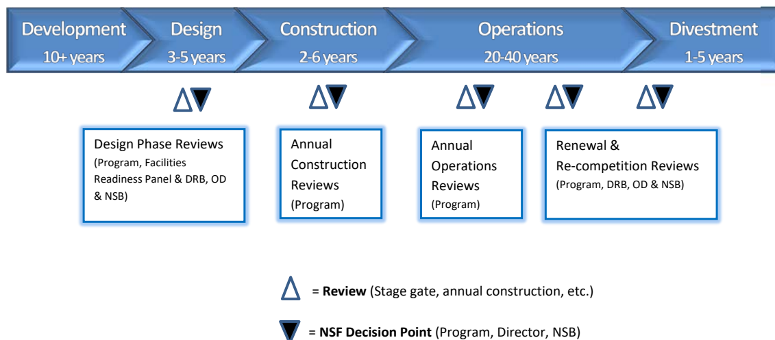
Figure 2.1.3-1 Progressive steps in the facility life cycle, showing the high-level review and decision points for exit and entry into each stage. The Design Stage is further broken down into phases.
