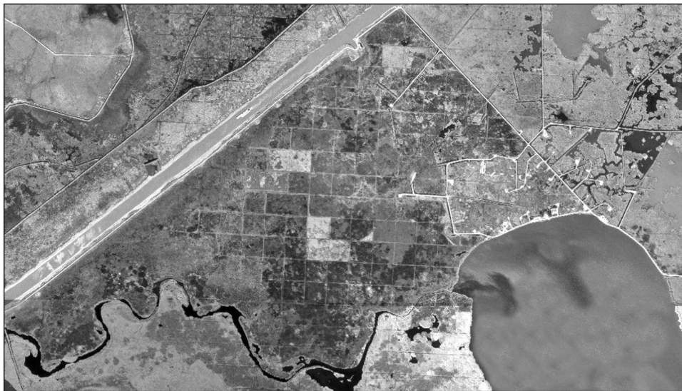
Figure 7: Compressed Marsh Grid from 3-D Seismic Study at McFaddin NWR (Tex.)
