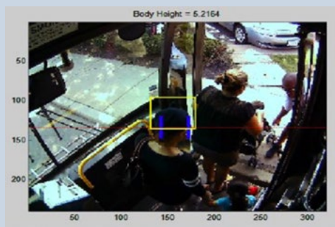
Figure 20 Counting Passengers through Body Height Curve
