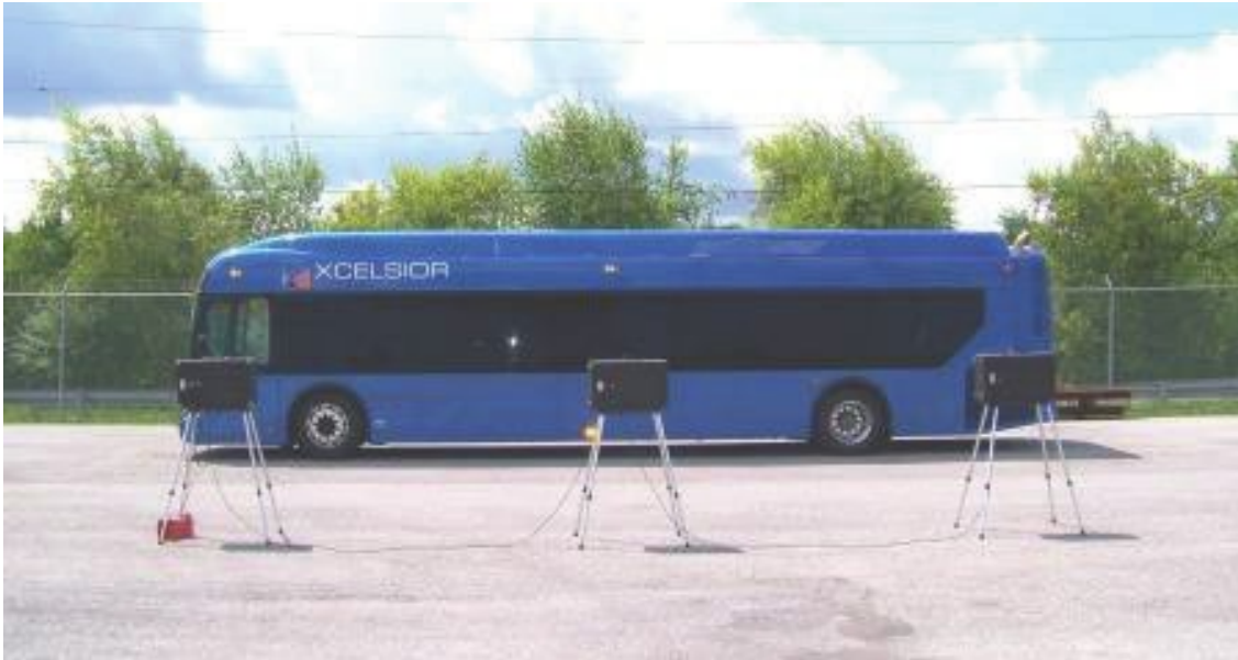
TEST BUS SET-UP FOR 80 dB(A) INTERIOR NOISE TEST
