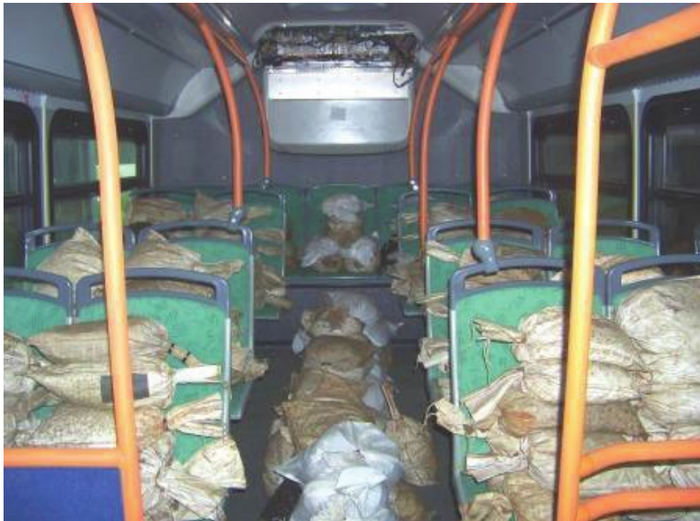
BUS LOADED TO 2.5 TIMES GVL (31,125 LBS)
