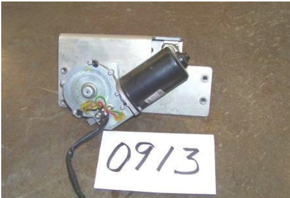
WIPER MOTOR REMOVAL AND REPLACEMENT (0.5 MAN HOURS)
