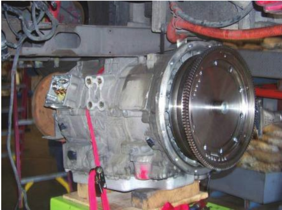
TRANSMISSION REMOVAL AND REPLACEMENT (18.0 MAN HOURS)
