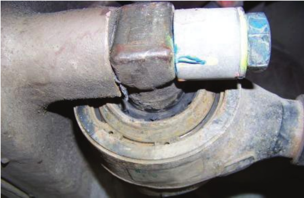
WORN BUSHING; RIGHT FRONT LOWER RADIUS ROD (4,273 TEST MILES)
