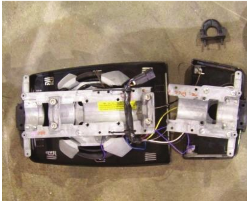
BROKEN REAR VIEW MIRROR MOUNTING BLOCK (4,815 TEST MILES)
