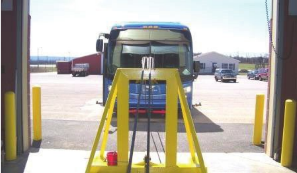
FRONT 20° UPWARD PULL
