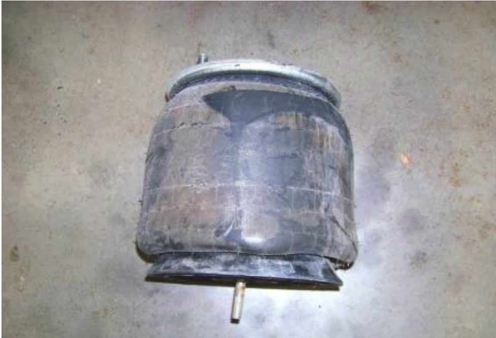
LEAKING LEFT FRONT AIR BAG (1,591 TEST MILES)
