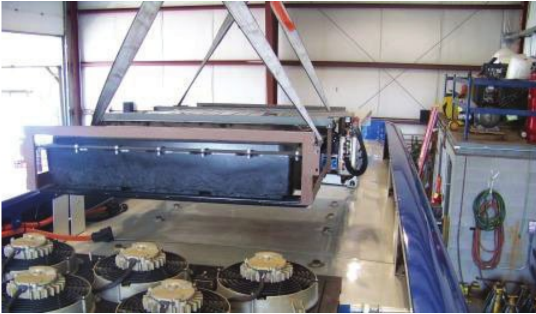
HYBRID BATTERY PACK REMOVAL AND REPLACEMENT (1.0 MAN HOURS)
