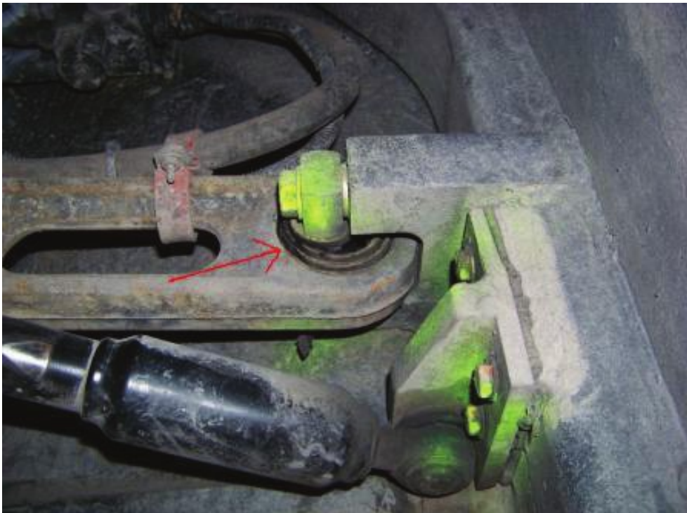
WORN BUSHING: RIGHT SIDE, UPPER RADIUS ROD (2,327 TEST MILES)
