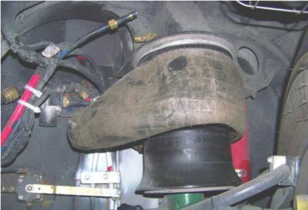
BLOWN OUT LEFT FRONT AIR BAG (4,815 TEST MILES)
