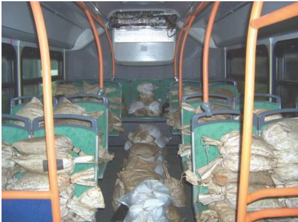
BUS LOADED TO 2.5 TIMES GVL (31,125 LBS)
