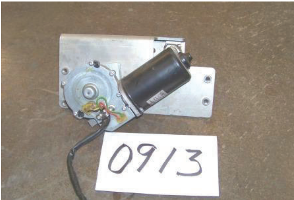
WIPER MOTOR REMOVAL AND REPLACEMENT (0.5 MAN HOURS)
