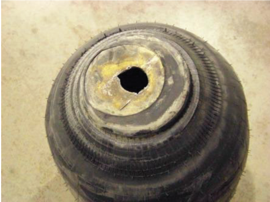
BOTTOM STUD BROKEN ON LEFT FRONT AIR BAG (13,516 TEST MILES)
