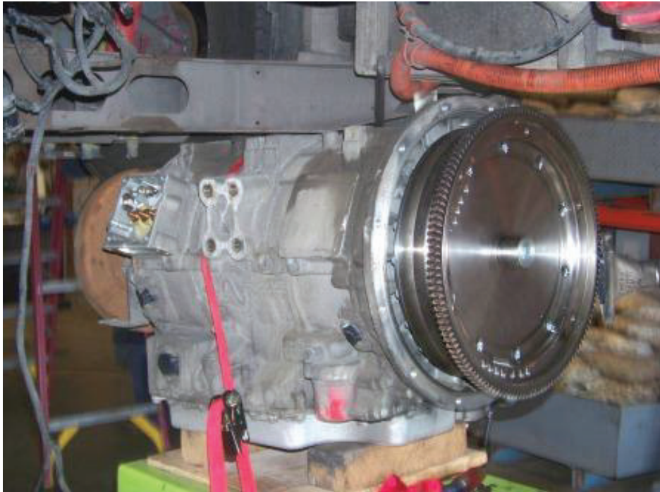
TRANSMISSION REMOVAL AND REPLACEMENT (18.0 MAN HOURS)
