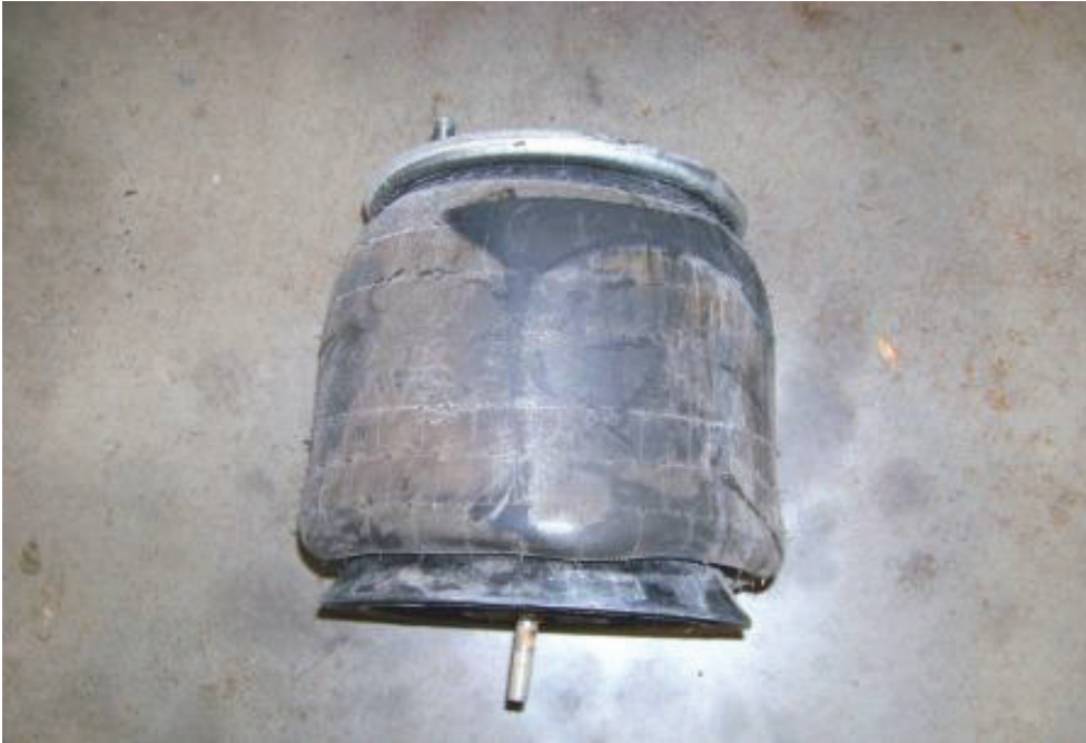
LEAKING LEFT FRONT AIR BAG (1,591 TEST MILES)
