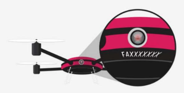
You must mark each aircraft with the assigned unique registration number before it is operated.
