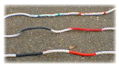
The 12" colored required marks can be accomplished in a variety of ways. Shown are three simple methods that were tested and found to work satisfactorily under normal conditions. At the top, colored twine is seized around the line and woven between the strands. In the center, the line was spray-painted; this method requires that the rope be dry. At the bottom, colored electrical tape was wrapped in one direction and then back over itself to form two layers.
