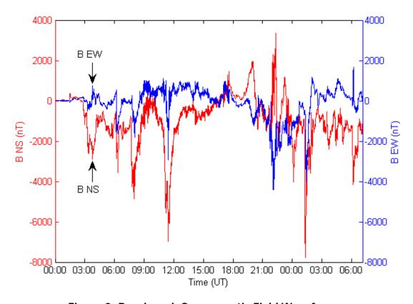
Figure 3: Benchmark Geomagnetic Field Waveform Red  $B_n$  (Northward), Blue  $B_e$  (Eastward)
