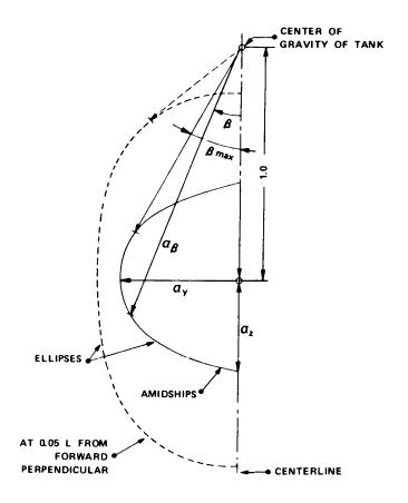
NOTE: RESULTING ACCELERATION (STATIC + DYNAMIC) =  $\alpha_{\beta}$ IN ARBITRARY DIRECTION  $\beta$ .
