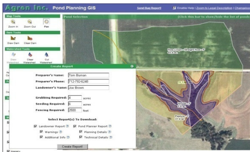
Figure 11. With a DEM, pond planning software took 15 minutes to develop 100+ design options for pond size/depth, dam height, drainage areas, pipe size, fencing costs, etc.
