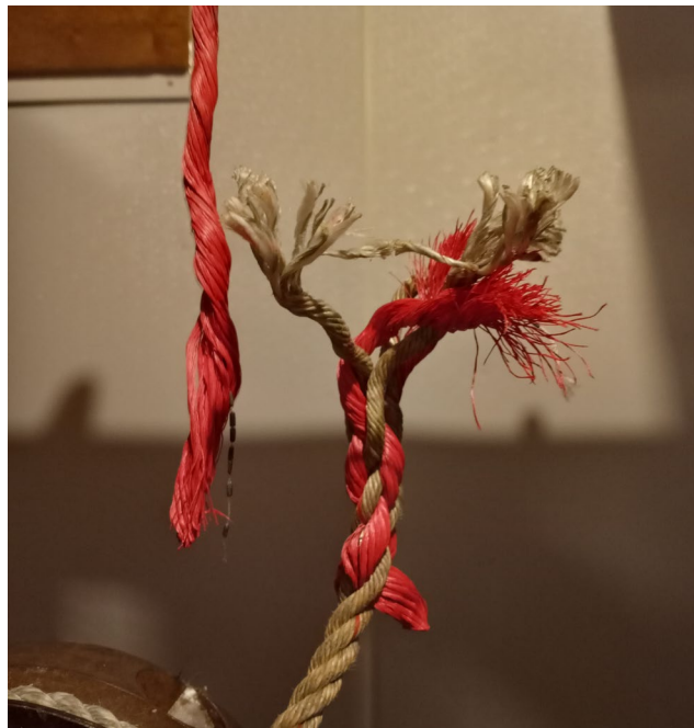
Figure 2: Picture of a 1700-lb weak rope on the rope breaking machine at ME DMR. This example shows a 1/2" weak rope (1700 lb) and 1/2" Everson sink, connected by a butt (or inline) splice. The weak rope broke at the connection point to the Everson sink line.
