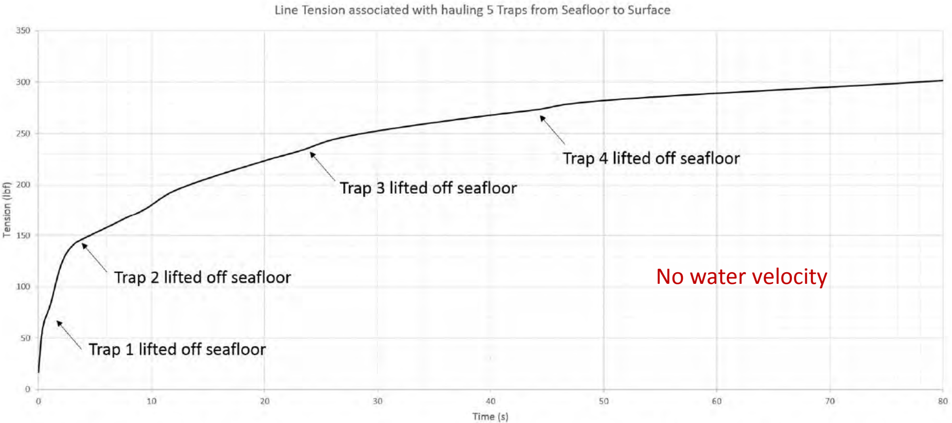
Figure 30: The line tension associated with a simulated recovery of a 5-lobster trap system, which initiated from the seafloor.
