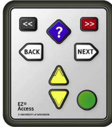
Figure 3: APC Kiosk EZ Access Keypad
