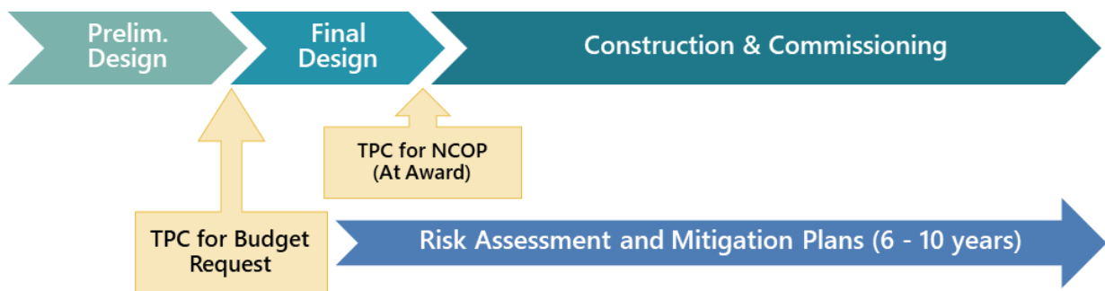
Figure 2.1.4-3 Linear Design-Construct Process is Classic "Waterfall Model" Implementation
