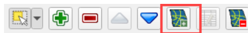
Figure 29. The Add Entity button on the Modify Area Feature dialog box toolbar
