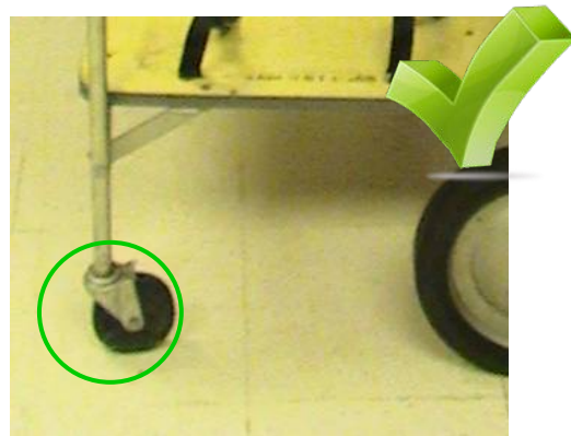
Figure 2 - Rollers pointed inward
