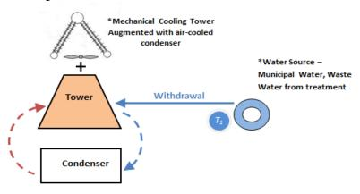
Withdrawal: Report the cooling tower makeup water that is removed from a water body.
