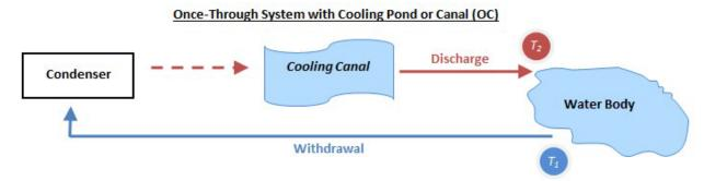
Withdrawal: Report the water that is removed from a water body for cooling, i.e. water used through the condenser.
