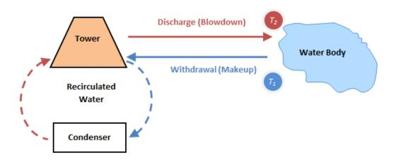
Withdrawal: Report the cooling tower makeup water that is removed from a water body.
