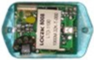
Data Storage tag (archival) | 1 x 3/4 inch | Black Sea Bass, Scup, Yellowtail Flounder, Cod
