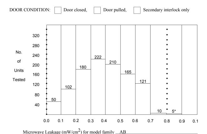
\*Reject limit exceeded by measurement at top edge of door frame because of excessive tolerance
