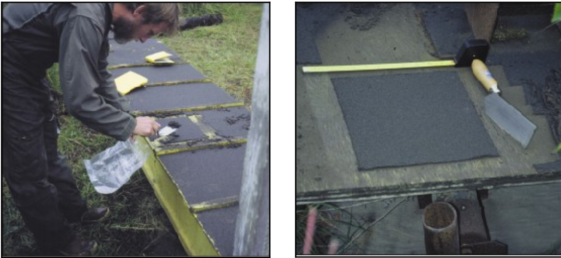
Figure 2. Collection of measured-area tephra samples from hard surfaces after 1992 eruption of Crater Peak/Mount Spurr, AK (photo from 9/21/92).
