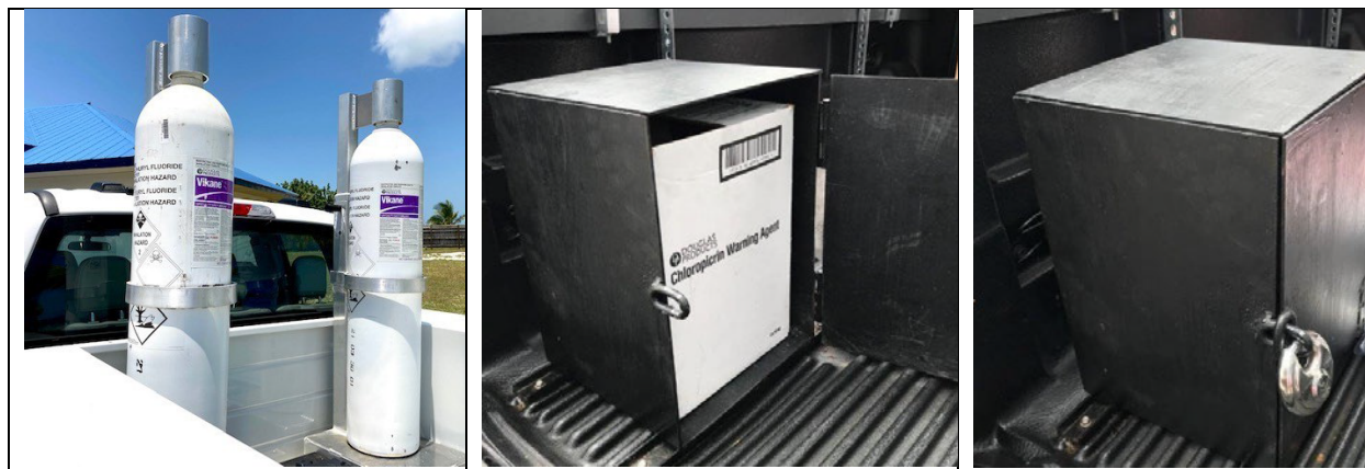
Fig. 2. Proper transportation of cylinders of Vikane ® gas fumigants (left) and chloropicrin container in HAZMAT packaging (center and right).
