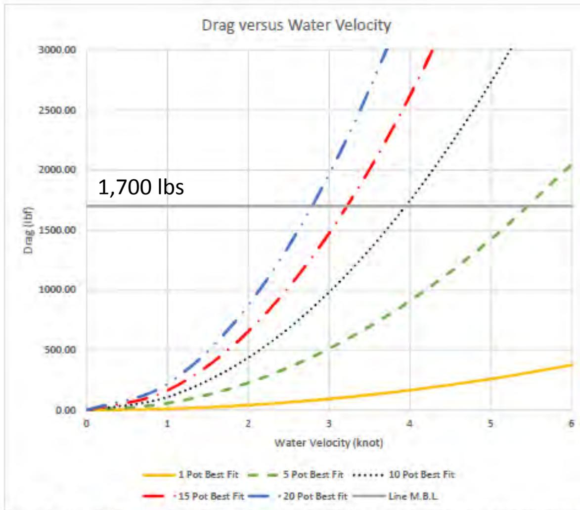
Figure 0: The velocity square best fit curves for a variety of lobster pot systems based on field data for a 1, 2 and 5 trap system. Each curve is governed by the equation shown in Table 4.
