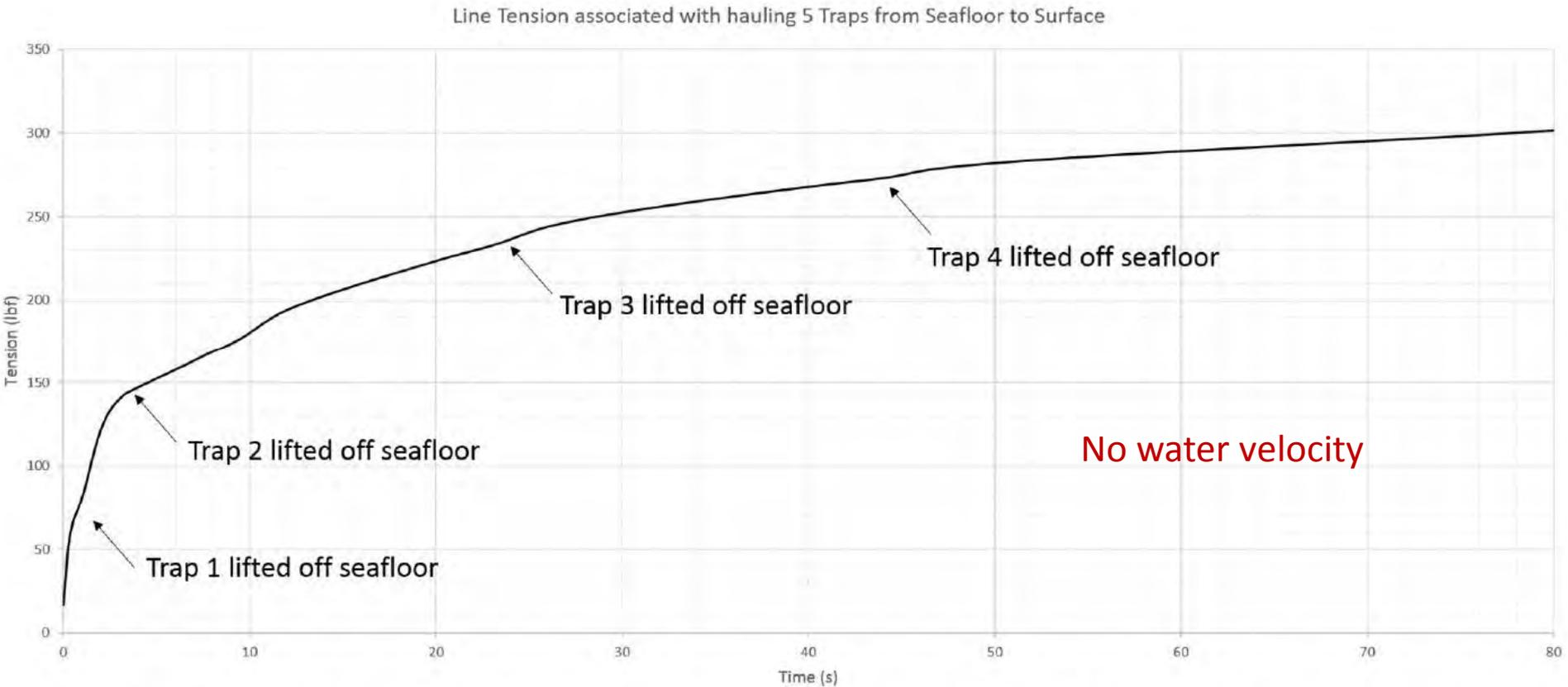
*Figure 30: The line tension associated with a simulated recovery of a 5-lobster trap system, which initiated from the seafloor.*
