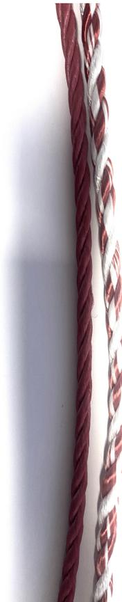
Ketcham Supply in New Bedford has been instrumental in getting these two 1700lb. weak ropes developed and manufactured. We are pleased to report that these weak ropes can be made in state specific colors and are hopeful that NMFS will utilize these weak ropes and various colorations for implementation as a default gear marking.
