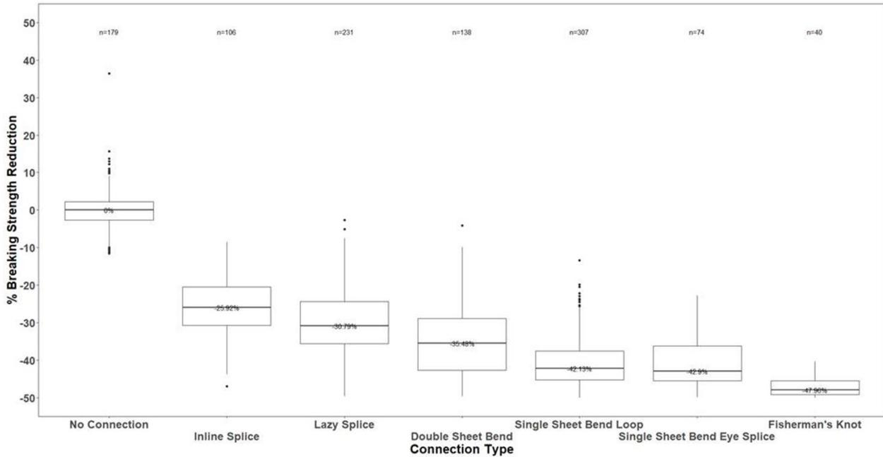
**Figure 1:** Percent reduction in break strength from rope breaking tests conducted by ME DMR. The samples include new rope from a variety of manufacturers, and in varying diameters. Reductions in breaking strength for various connection point types, as well as a segments of rope with no connections, are shown. Reduction in breaking strength was measured from the breaking strength of the weakest rope in the configuraton.
