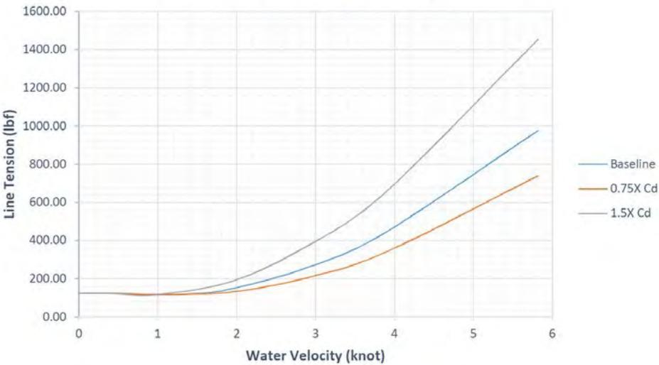
Trap drag coefficient and # of traps on the water column had the most sensitivity as water velocity increases
