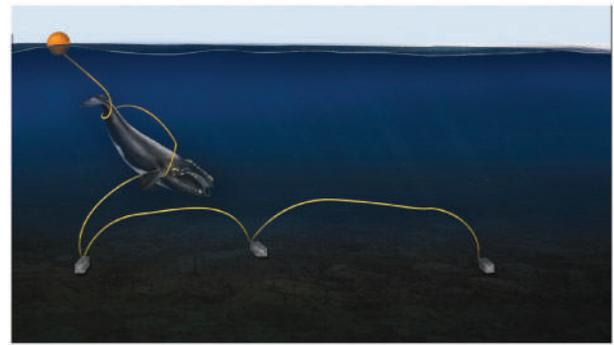
**Figure 5.** Illustration of a string of bottom traps (known as a trawl), linked by negatively buoyant ground lines, with a line from the end trap to a surface marker buoy. Filter-feeding North Atlantic right whales risk open mouth and appendage entanglements when swimming in fields of these vertical lines and buoys.
