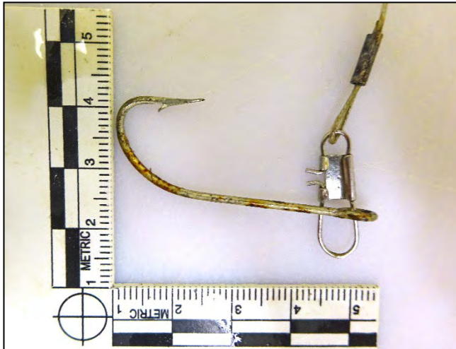
Configuration photos: Take closer images of all aspects of the material to clearly show how they are attached or arranged. Always include an internal ruler or scale.
