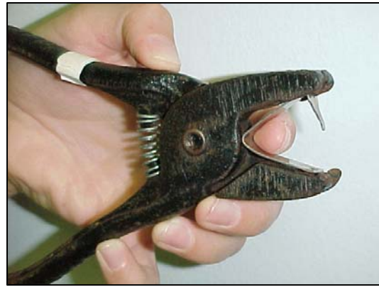
Figure 6-2. Inserting the tag into the applicator (NMFS/SEFSC photo).
