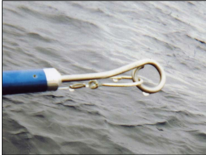
Figure 2-6. Point of the hook is shielded to prevent re-engagement (NMFS/SEFSC photo).
