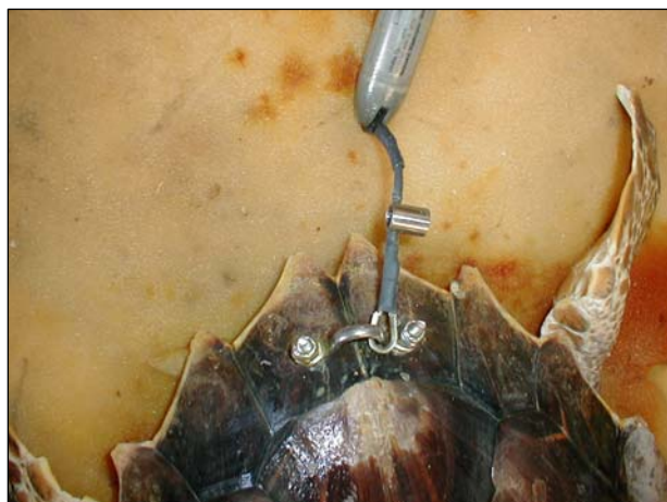
Figure 7-1. Attachment of an archival satellite tag on a hardshell turtle (NMFS/SEFSC photo).
