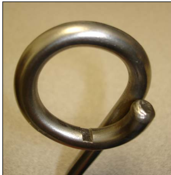
Figure 2-7 a, b and c. Notch the pigtail curl where the shank of the hook contacts the vertical bottom of the pigtail curl, \sim 1/16'' - 1/8'' deep and \sim 1/8'' wide using a metal file [(a) Photo courtesy of ARC; (b) and (c) NMFS/SEFSC photos].
