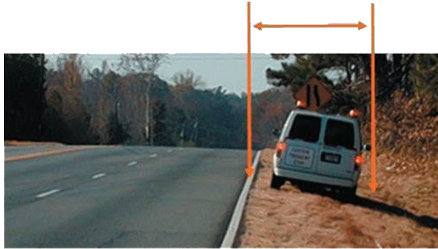
Figure 31: Earth Shoulder Measurement
