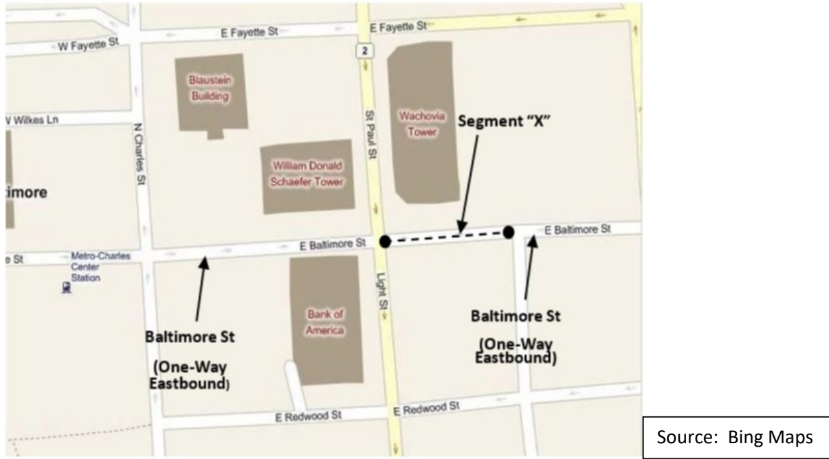
Figure 9: One-Way Roadway (Code 1) Example
