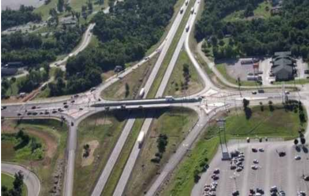
Figure 61: Full Access Control (Code 1) Examples All access via grade-separated interchanges
