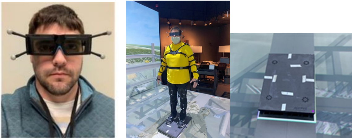
Virtual reality glasses to detect eye movement and head sway (left). Heart rate monitor to collect changes in heart rate during participation (middle); and force plate with biomarkers to detect balance and postural sway during participation (right).
