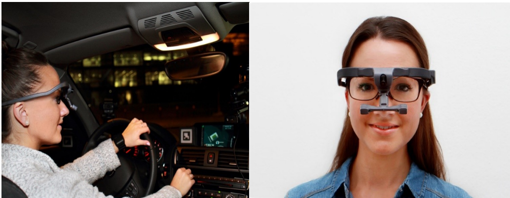
Illustrations of Dikablis eye trackers being worn by the participant in a stationary vehicle while responding to virtual reality simulations on TV monitors.
