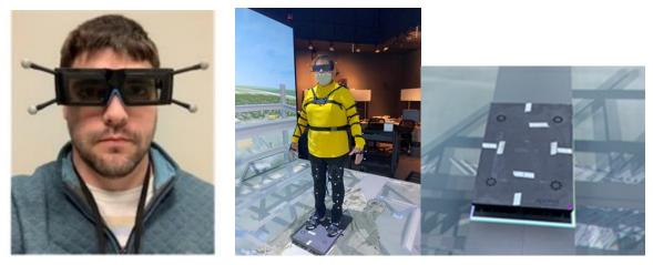
Virtual reality glasses to detect eye movement and head sway (left). Heart rate monitor to collect changes in heart rate during participation (middle); and force plate with biomarkers to detect balance and postural sway during participation (right).
