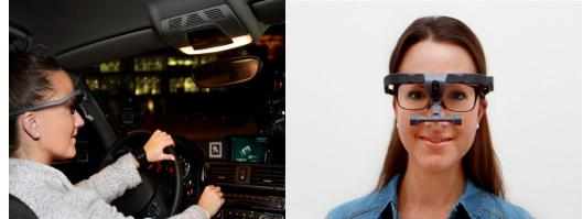
Illustrations of Dikablis eye trackers being worn by the participant in a stationary vehicle while responding to virtual reality simulations on TV monitors.
