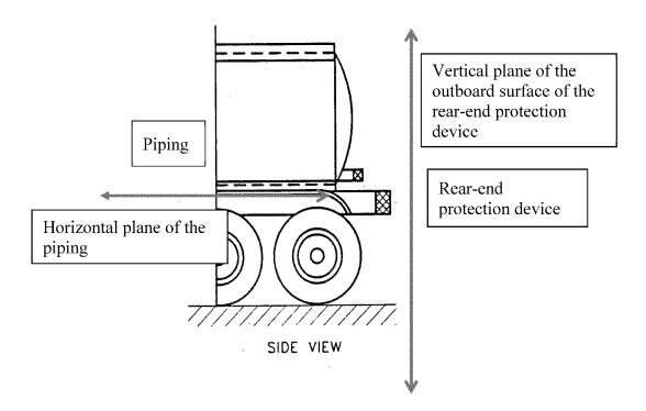
Paragraph (d)(2) indicates the dimension requirements for the rear-end cargo tank protection device. Paragraph (d)(3) specifies additional design requirements for the rear-end protection device and its attachments on DOT Specification 406, 407, and 412 cargo tank motor vehicles. In paragraphs (d)(2)(i)–(iii) and (3), PHMSA proposes to spell out the dimensions instead of using a numerical value, for grammatical correctness.
