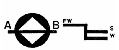
(c) Where the Special Service Load Line Certificate is issued in addition to an Unlimited Coastwise or International Load Line Certificate, the wording of the Special Service Load Line Certificate is to be identical to that given in paragraph (a) of this section, but the markings indicated in the form shall be replaced by the following markings:
