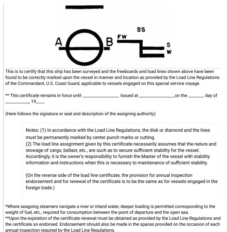
(b) Where the Special Service Load Line Certificate is issued in addition to a Great Lakes Load Line Certificate, the wording of the Special Service Load Line Certificate is to be identical to that given in paragraph (a) of this section, but the markings indicated in the form shall be replaced by the following markings:
