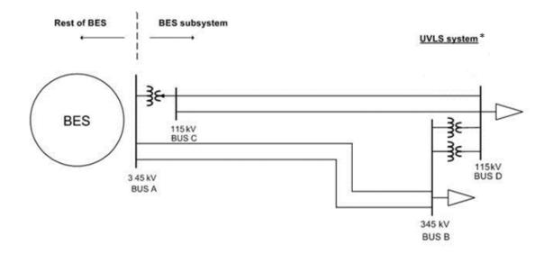
\*UVLS systems may be installed at either, or both, bus B and D
