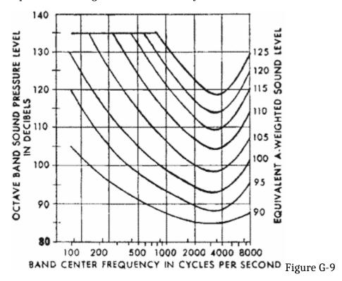
Equivalent sound level contours. Octave band sound pressure levels may be converted to the equivalent A-weighted sound level by plotting them on this graph and noting the A-weighted sound level corresponding to the point of highest penetration into the sound level contours. This equivalent A-weighted sound level, which may differ from the actual A-weighted sound level of the noise, is used to determine exposure limits from Table 1.G-16.
