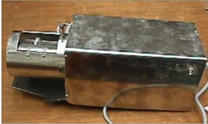
*Figure 23 – Mechanical stainless steel oyster grinder*
