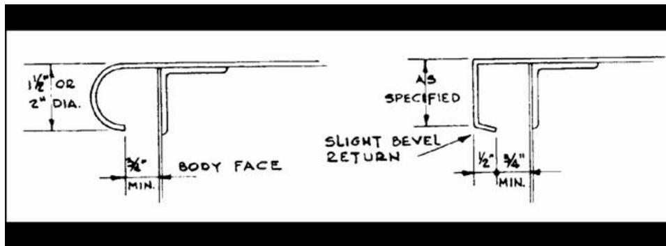
*Figure 19 – Exposed edges and nosings on horizontal surfaces*
