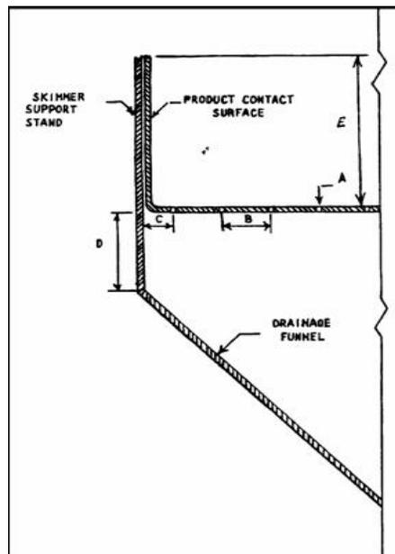
**Figure 13** – Skimmer cross sectional side view
