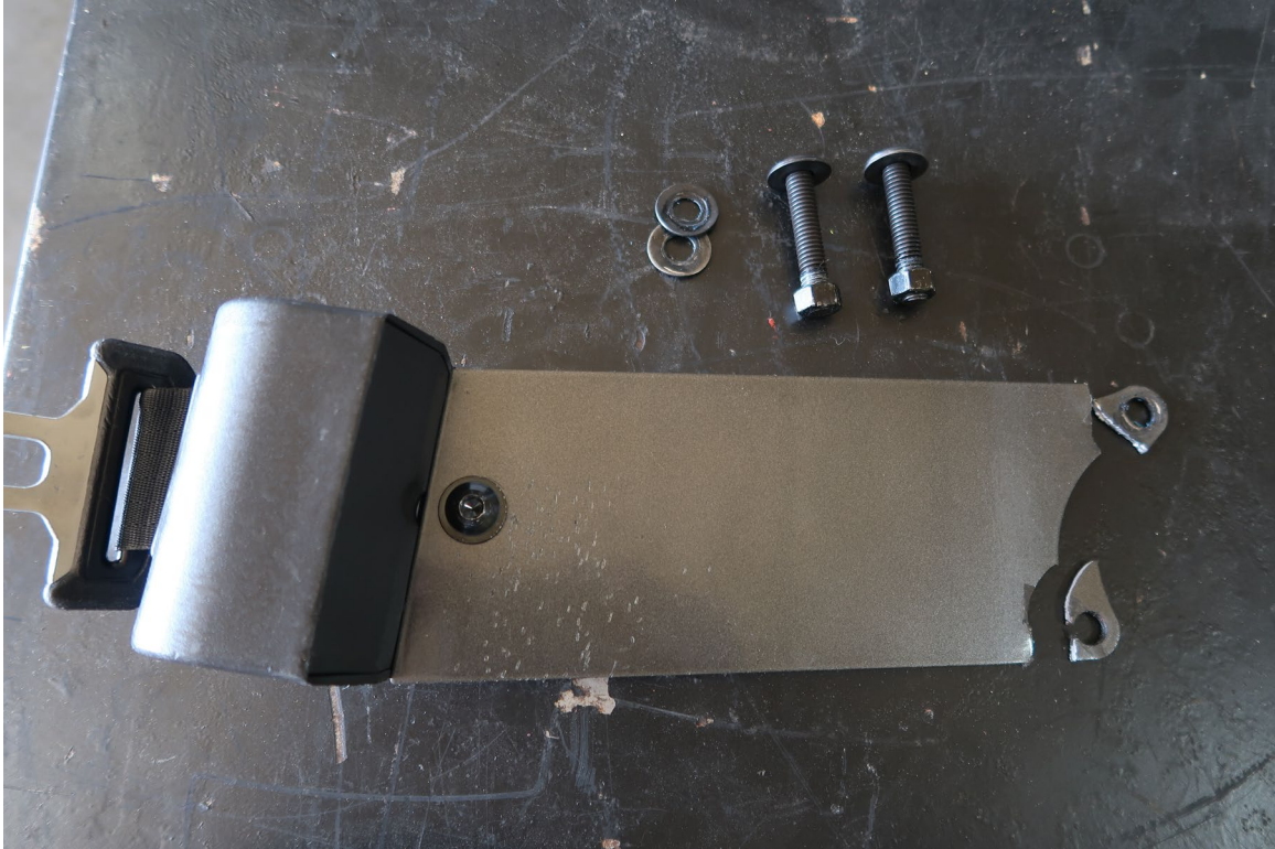
SEATBELT BRACKET FOR ADA LIFT IS BROKEN (4,298 TEST MILES)
