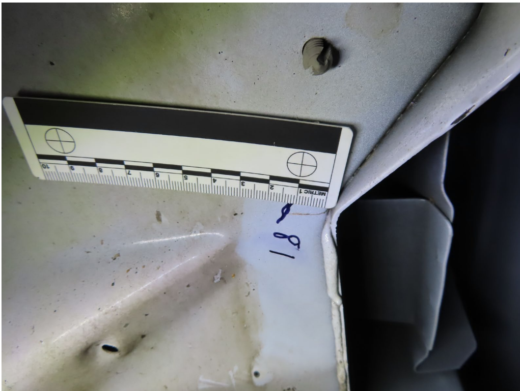
CRACK #18; CRACK ON STREETSIDE INNER FENDER WELL BEHIND PLASTIC LINER ABOVE THE TIRE
