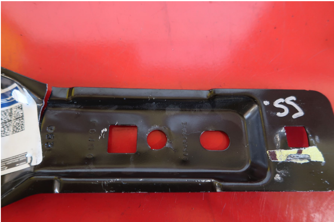
STREETSIDE GRILLE SUPPORT BRACKET IS CRACKED (3,817 TEST MILES)
