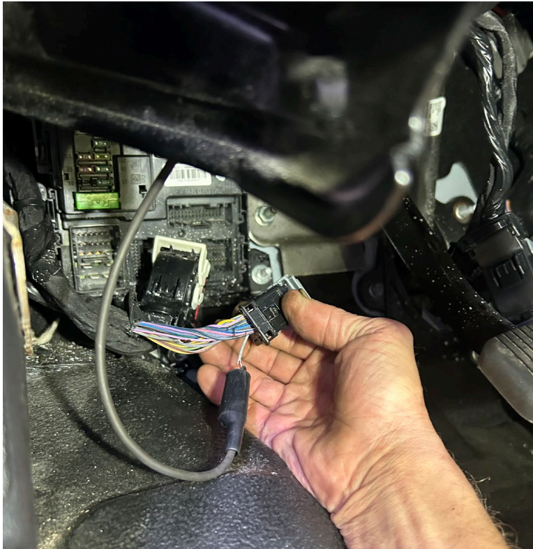
BROKEN WIRE IN THE WIRING HARNESS (2,268 TEST MILES)
