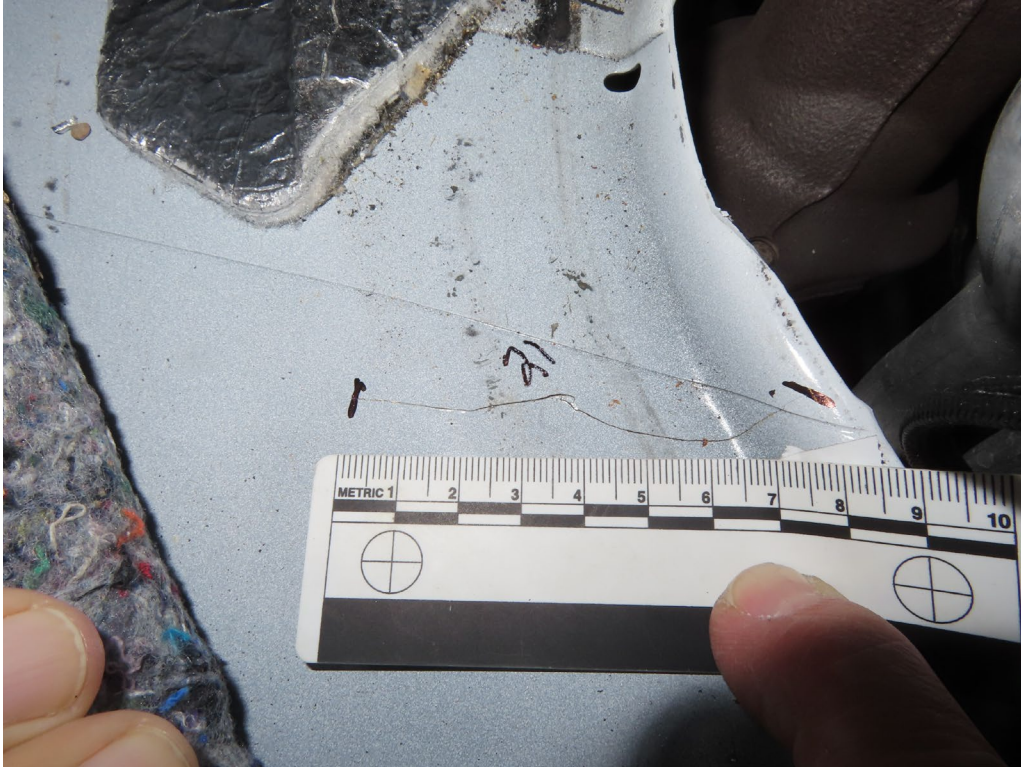
CRACK #21; CRACK ON THE STREETSIDE DRIVER FLOOR AREA
