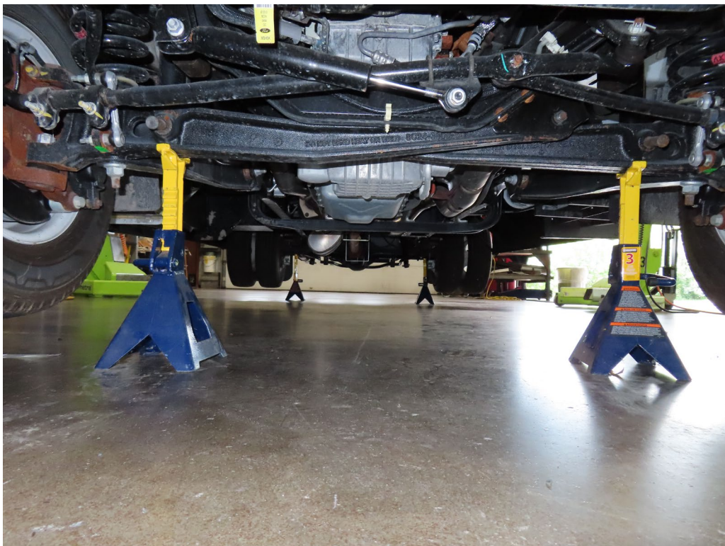
JACK STANDS IN PLACE – FRONT AND REAR
