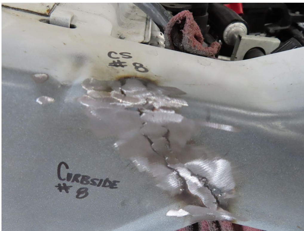
CRACK #8 – WELDING REPAIR (4,750 TEST MILES)
