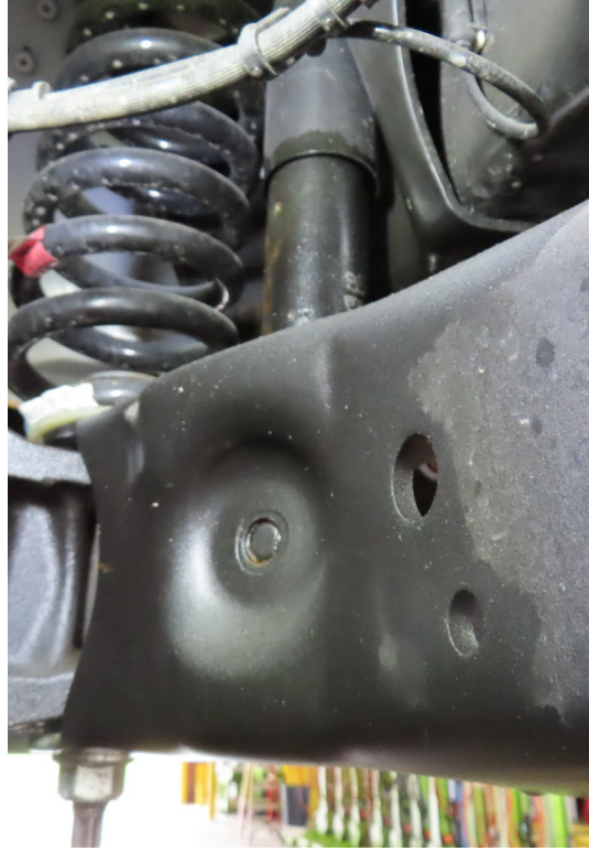
FRONT, STREETSIDE SHOCK ABSORBER IS LEAKING (334 TEST MILES)
