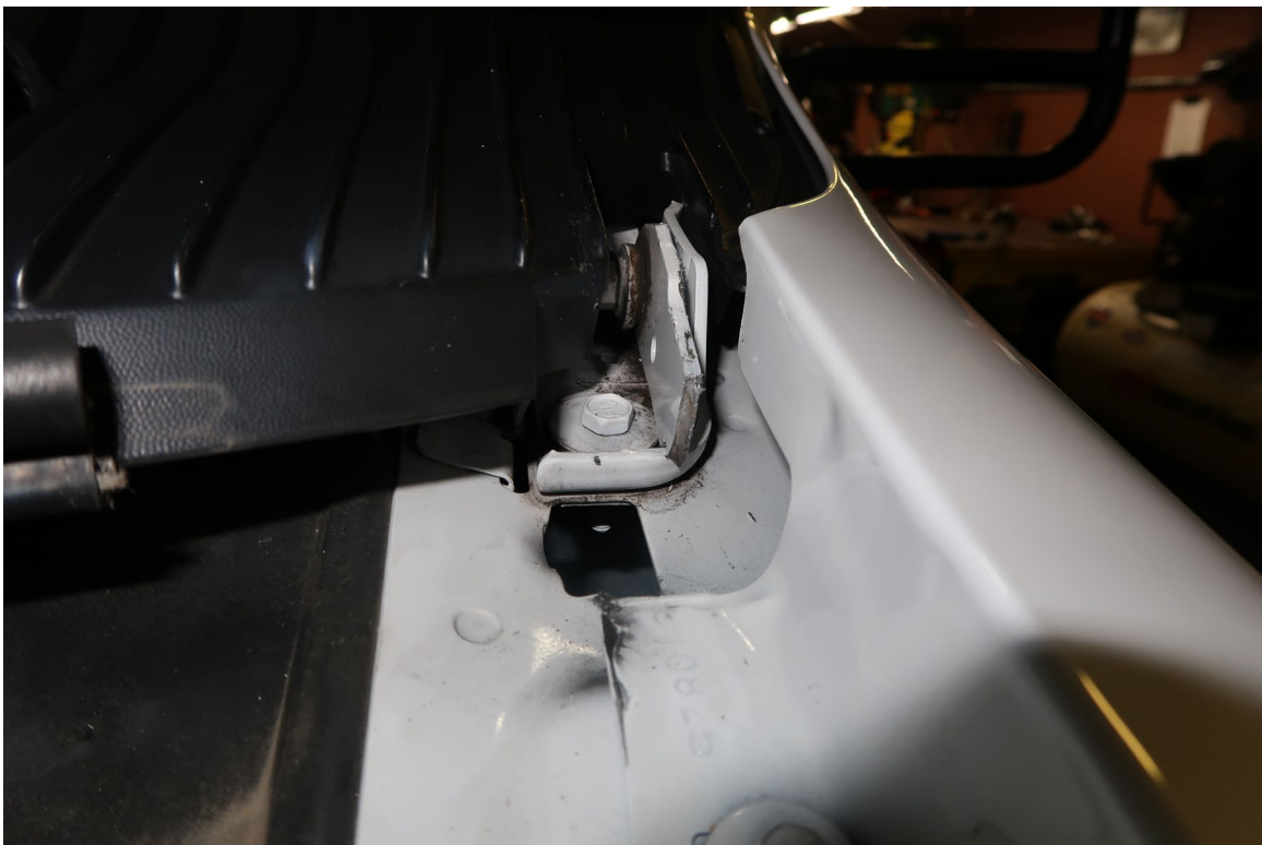
STREETSIDE HOOD HINGE IS BROKEN (6,356 TEST MILES)
