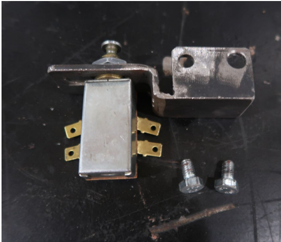
ADA DOOR SWITCH REPLACED WITH MODIFIED VERSION; OLD SWITCH (LEFT), NEW SWITCH (RIGHT) (4,457 TEST MILES)
