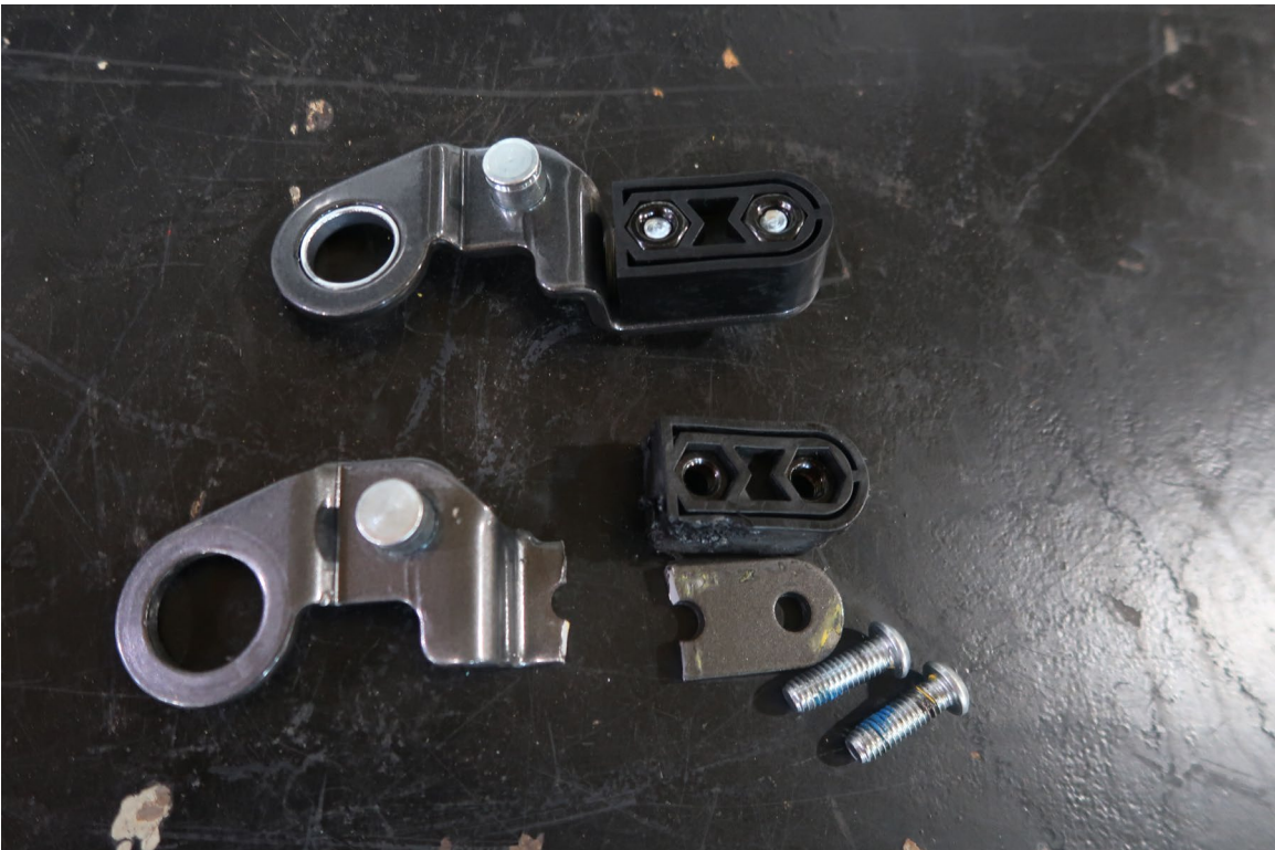
CURBSIDE, REAR ADA LIFT INBOARD BARRIER BRACKET IS BROKEN (4,298 TEST MILES)
