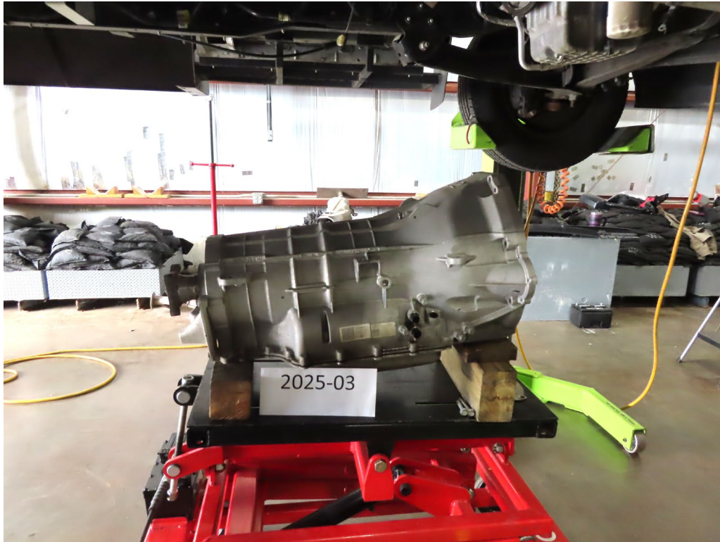
TRANSMISSION REMOVAL AND REPLACEMENT (6.50 LABOR HOURS)
