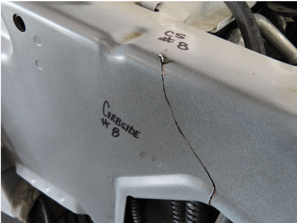
CRACK #8 – CRACK IN CURBSIDE INNER FENDER (4,750 TEST MILES)
