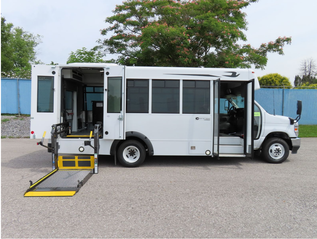
THE BRAUN CORPORATION NCL1000F1B3454HB-2 ELECTRIC FOLD DOWN ADA LIFT
