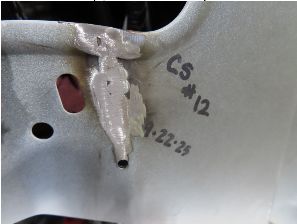
CRACK #12 – WELDING REPAIR OF CRACK IN INNER FENDER (4,750 TEST MILES)
