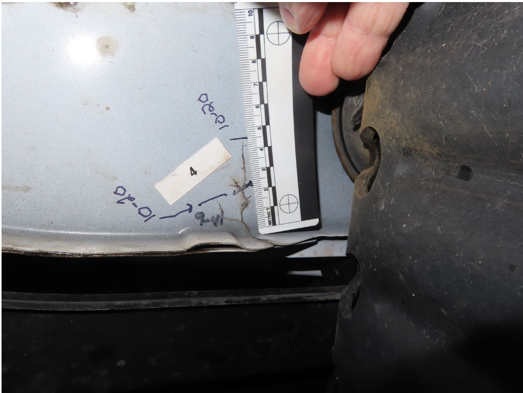
CRACK #4; CRACK UNDER FRONT CORE SUPPORT ON STREETSIDE IN FRONT OF STREETSIDE FRONT WHEEL
