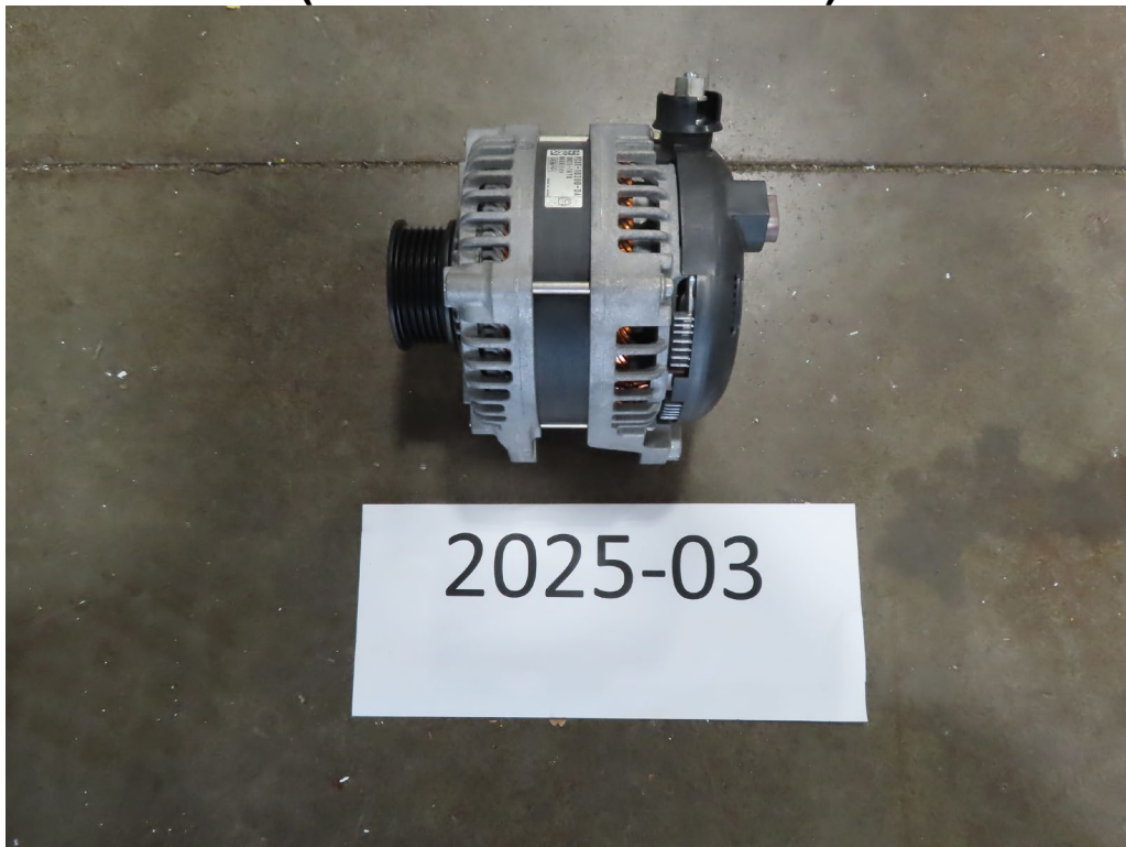
ALTERNATOR REMOVAL AND REPLACEMENT (1.00 LABOR HOURS)
