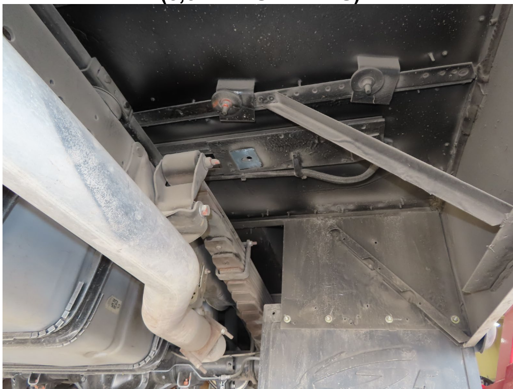
ADA MOUNTING BOLT BROKE AND FELL OUT (6,008 TEST MILES)
