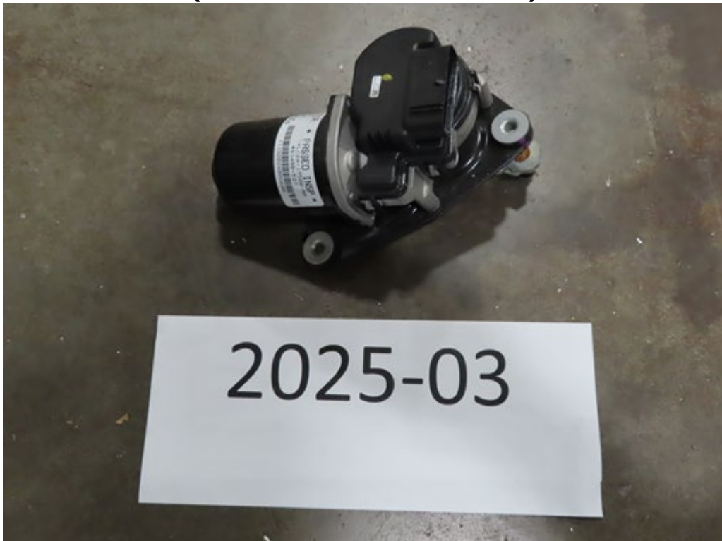
WIPER MOTOR REMOVAL AND REPLACEMENT (0.50 LABOR HOURS)
