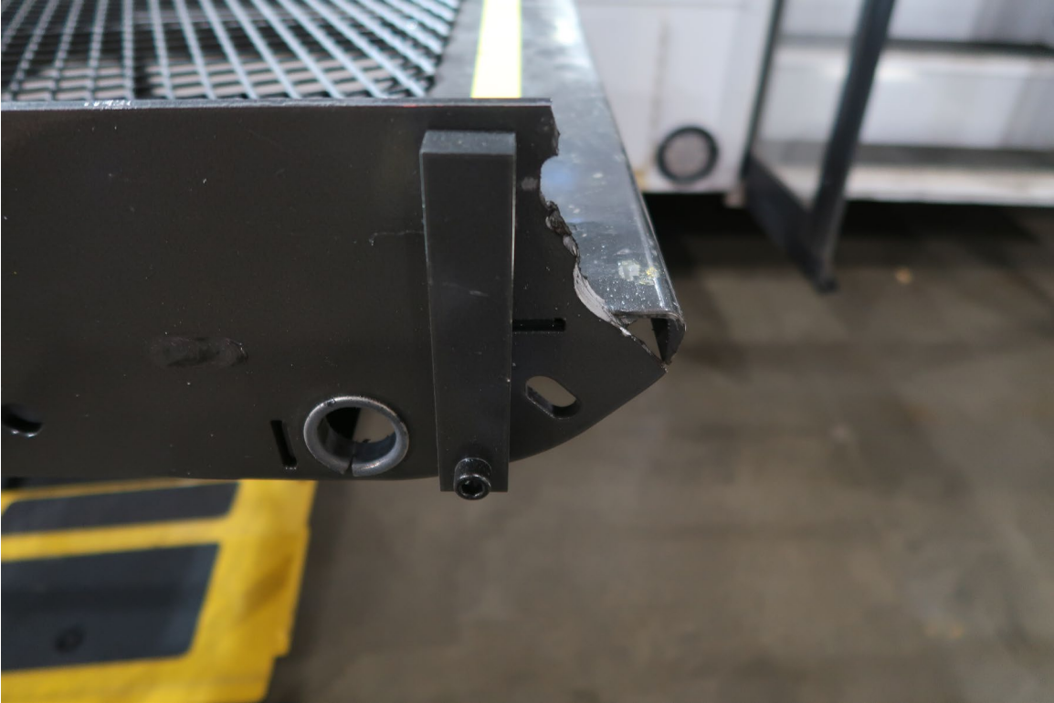
WHEELCHAIR PLATFORM BROKEN WHERE THE INNER BARRIER ATTACHES (6,540 TEST MILES)
