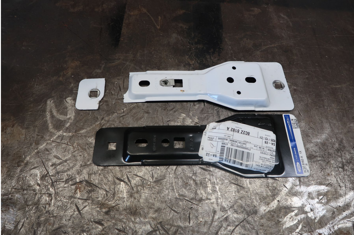
CURBSIDE GRILLE SUPPORT BRACKET IS CRACKED (2,930 TEST MILES)
