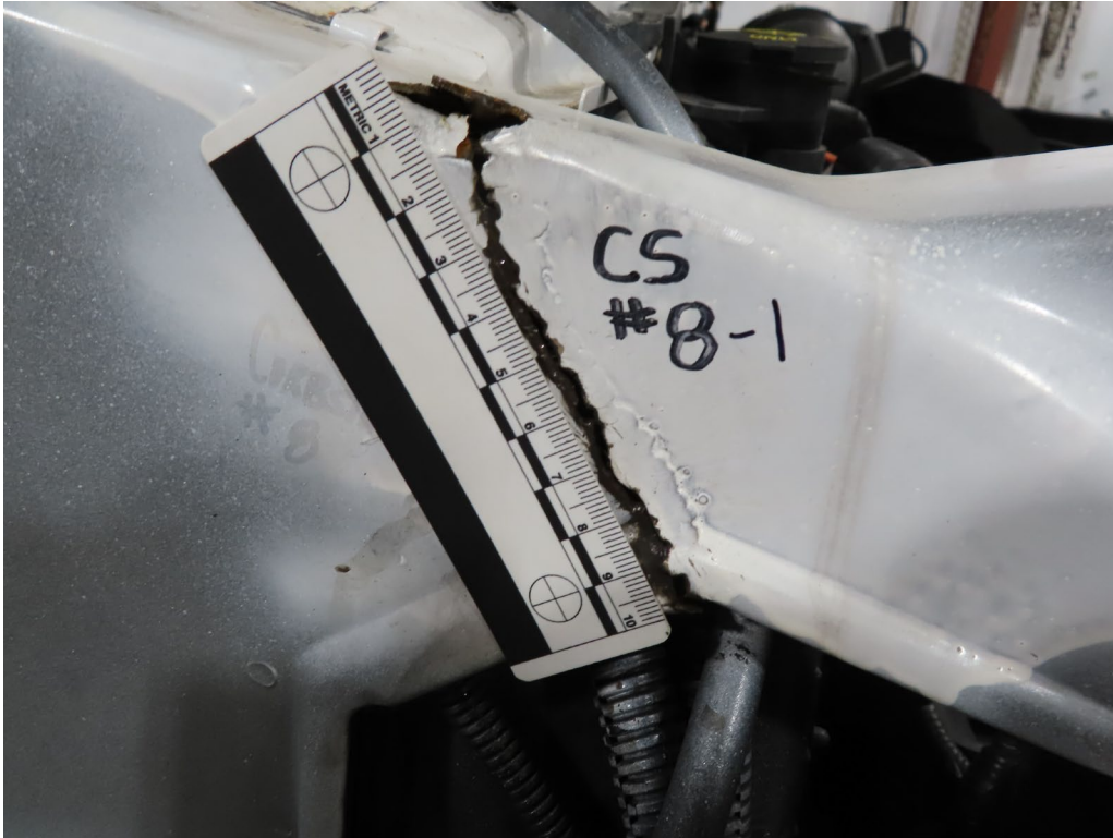
CRACK #8-1; WELDED REPAIR OF CRACK #8 ON THE CURBSIDE INNER FENDER UNDER THE HOOD HAS CRACKED
