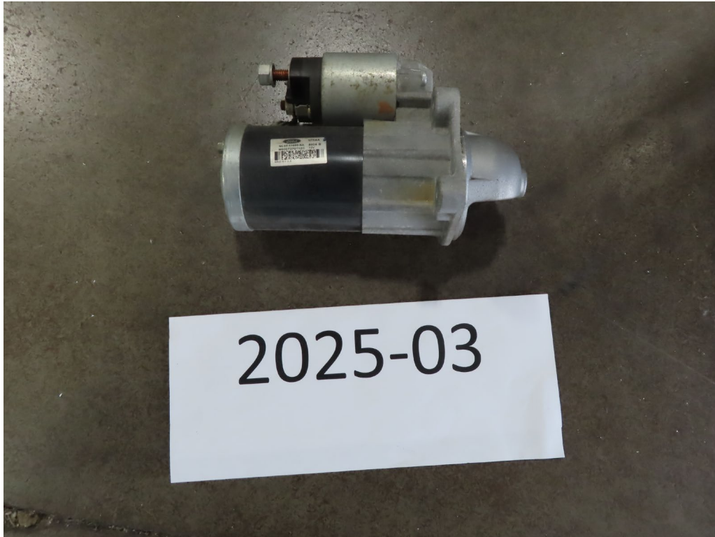
STARTER REMOVAL AND REPLACEMENT (0.67 LABOR HOURS)
