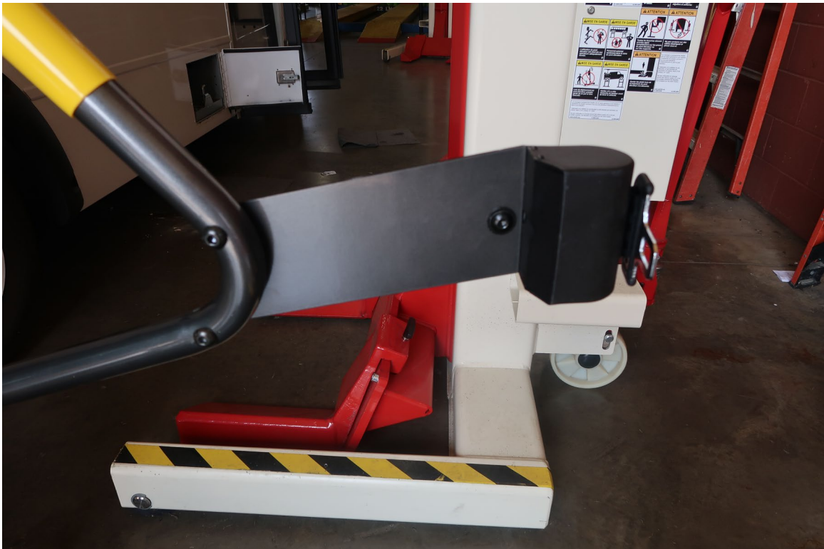
SEATBELT BRACKET FOR ADA LIFT WAS REPLACED (1,815 TEST MILES)
