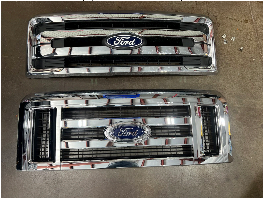
GRILLE REPLACED; TOP IS ORIGINAL, BOTTOM IS REPLACEMENT (4,345 TEST MILES)
