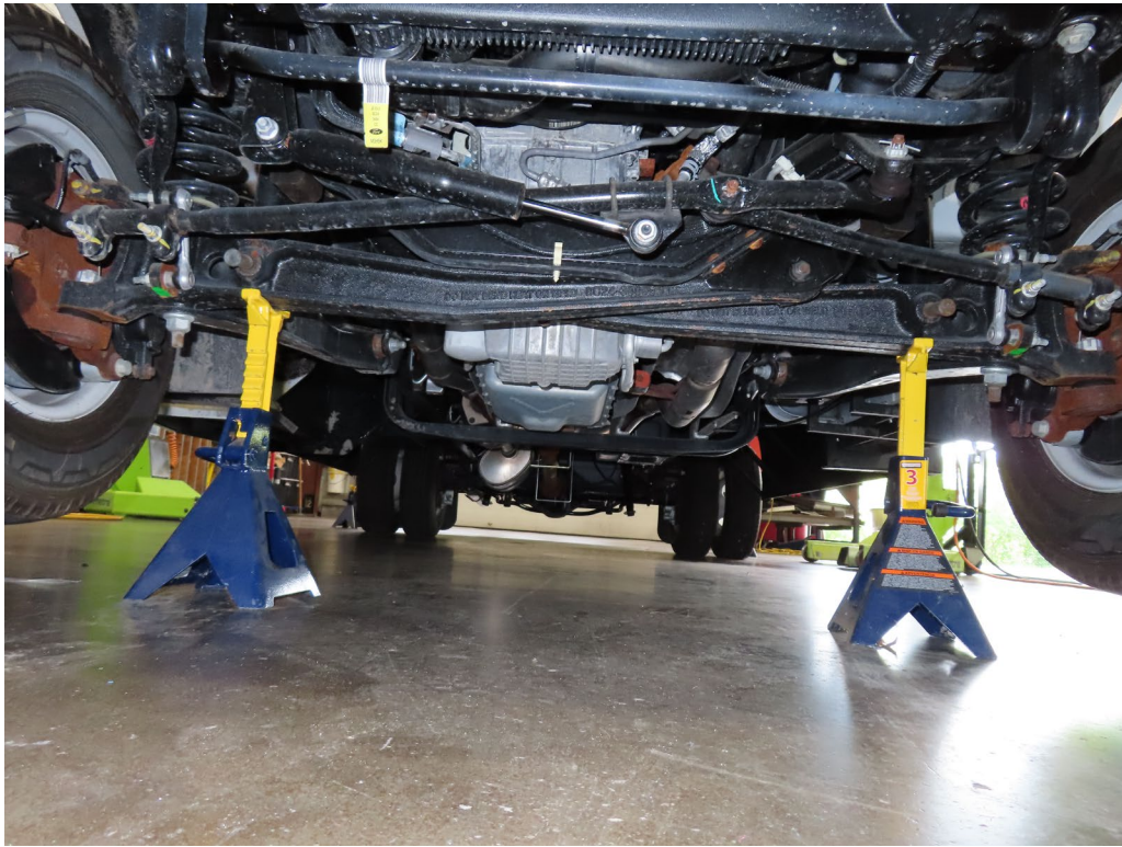
JACK STANDS IN PLACE - FRONT
