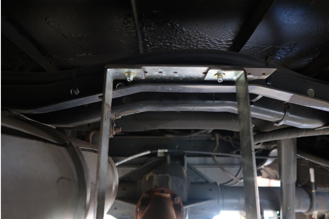
RIVETS REPLACED ON THE REAR MOST DRIVESHAFT LOOP (2,930 TEST MILES)
