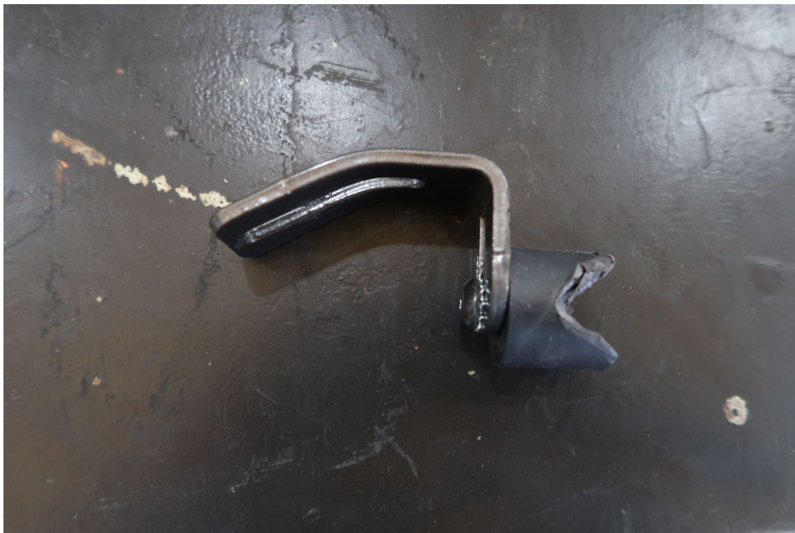
ADA RAMP STOP BRACKET IS BROKEN (5,512 TEST MILES)
