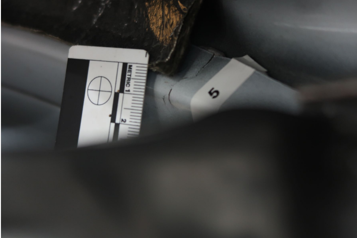
CRACK #5; CRACK IN CURBSIDE INNER FENDER STRUCTURE IN FRONT OF CURBSIDE FRONT ENTRANCE STEPS
