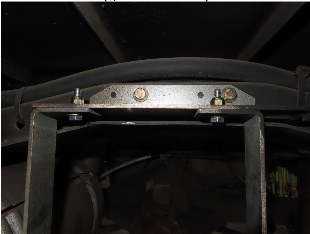
RIVETS ON THE REAR MOST DRIVESHAFT LOOP REPLACED WITH BOLTS, WASHERS AND LOCK NUTS (5,512 TEST MILES)
