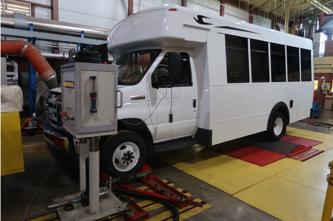
BUS TESTED ON CHASSIS DYNAMOMETER FOR PERFORMANCE, FUEL ECONOMY AND EMISSIONS
