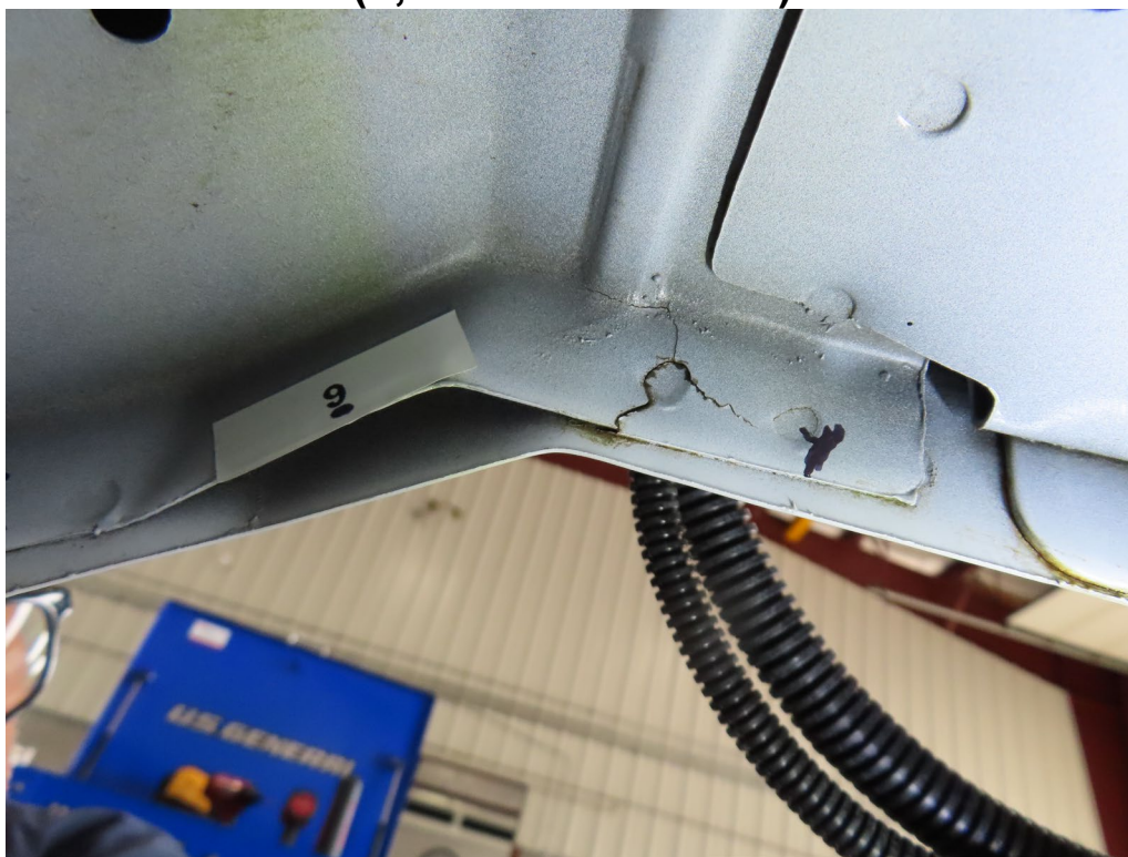
CRACK #9 – CRACK IN INNER FENDER STRUCTURE ABOVE CURBSIDE FRONT TIRE (4,750) TEST MILES
