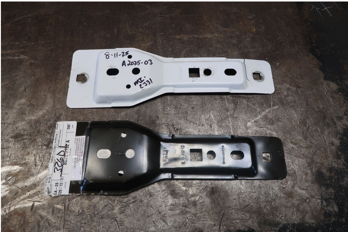
STREETSIDE GRILLE SUPPORT BRACKET IS CRACKED (2,282 TEST MILES)
