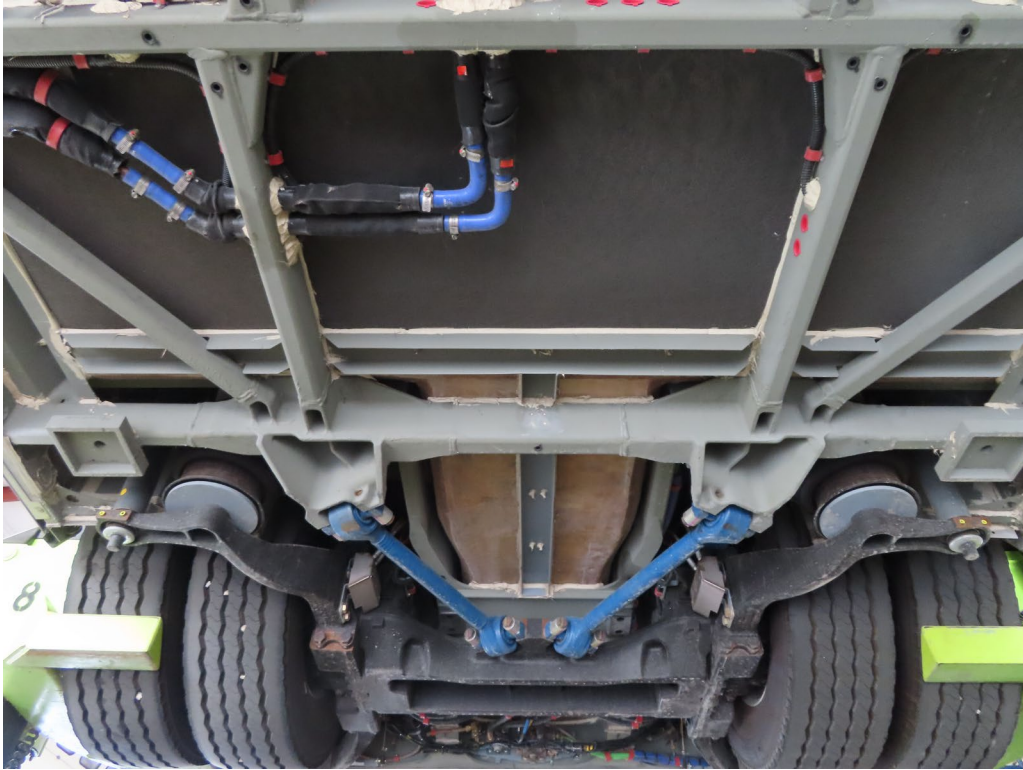
UNDERSIDE OF BUS – MIDDLE DRIVE AXLE
