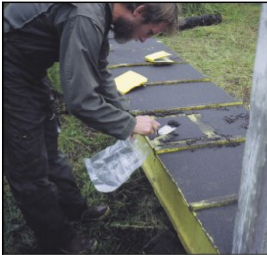
Figure 2. Collection of measured-area tephra samples from hard surfaces after 1992 eruption of Crater Peak/Mount Spurr, AK (photo from 9/21/92).
